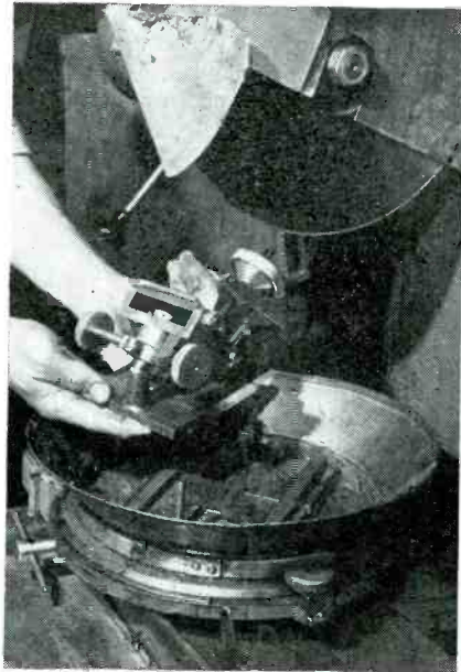
Quartz cutting jig ready for positioning on the movable table beneath the cutting saw
